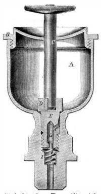
were omitted altogether. The rapidity of the discharge may be regulated by turning the spindle and screwing the plug, E, up or down. The spring, I, is used to prevent the jar of the machinery or any slight accidents from causing the plug, D, to become displaced when once adjusted.
