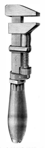
B, on the end of the handle, it is better to make the wrench as shown in this engraving. Here the screw step, A, is carried by the shank, C, of the wrench, thus giving great stiffness and rigidity to the jaws and rendering them more capable of retaining a firm hold on a nut. The step of this wrench is made separate, and fits tightly to the shank, where it is retained by a stout screw thimble, D.
