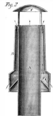
et, B, and a hood, C, as shown in Figs. 1 and 2. The lower part of the jacket is enlarged, as at D, and has openings, E, through which the air enters. It issues at the top, as shown. The jacket is supported by braces, F, at top and bottom. The air circulating through this appurtenance creates a current within the main pipe, A, which causes the fire to burn briskly. It would seem to be a useful invention.
