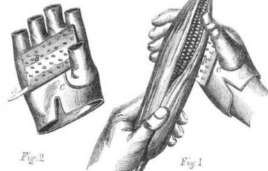
This glove can be used for husking as well | readily pulled down, the glove protecting the as shelling corn. A plate, B, of leather, metal, or any other suitable material, armed with pins as teeth, is secured to the palm of the glove or mitten, C. In our engraving, Fig. 1 represents the husking operation, which is performed by grasping the butt-end of the ear with the left hand, and pressing the right hand, on which is the glove, against the small end of the husk, and by slightly turning the
