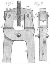
c, around which they can rotate, and as this is not in the center of B, by turning them round, they will accommodate different sized articles; these corresponding sides may be numbered as shown in our illustration, so that they may easily be brought in unison. By their being able to revolve, they can easily grasp a substance of any angle, and although the principle is especially intended for blacksmith's tongs, it is applicable to many other purposes and tools.
