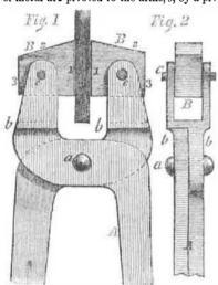
c, around which they can rotate, and as this is not in the center of B, by turning them round, they will accommodate diffierent sized articles; these corresponding sides may be numbered as shown in our illustration, so that they may easily be brought in unison. By their being able to revolve, they can easily grasp a substance of any angle, and although the principle is especially intended for blacksmith's tongs, it is applicable to many other purposes and tools.
