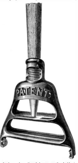
A, having a sharp-threaded screw on the inside to receive the handle; the other piece is made with a yoke or ring, B, which passes over the socket. The handle is made a little tapering and pointed at the end. By inserting it, when the clamp is closed, through the yoke into the socket, and turning it round, the screw in the socket cuts a thread on the handle, which secures it very firmly, and, at the same time, fastens the clamp and compresses the filling.
