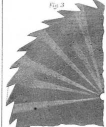
be filed up sharp, finishing with a fine, singlecut file. The cutting edge of each tooth should be parallel with the center of the mandrel, and the front and back of the teeth kept on the lines as described, and shown in Fig. 3. Mill saws, with teeth such as are shown in Fig. 4, after being straightened on the edge,
