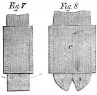
bound together with the iron band, C. It is used to widen the points of saw teeth when they-have become worn and blunted on the corners, and may be used without the necessity of filing the saw afterwards.
