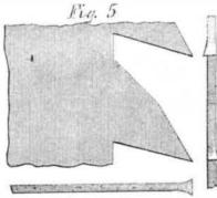
edge, the teeth are filed sharp at the points, like a cross-cut saw, alternately highest on the outside, and then upset with the punch.
