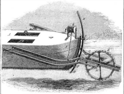
onward, somewhat in a manner analogous to the motion of a locomotive. The frame allows the wheel to rise and fall to accommodate itself to the inequalities of the bottom.
