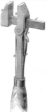
tionable propriety, be termed the fixed jaw. F is a pin, by which E is secured to B. G is the movable jaw, and G' a sufficiently long rectangular shank, which passes freely through a corresponding opening in E. The lever, D, is urged by the spring, C, into such position that it pinches and holds the shank, G', very firmly in its position.
