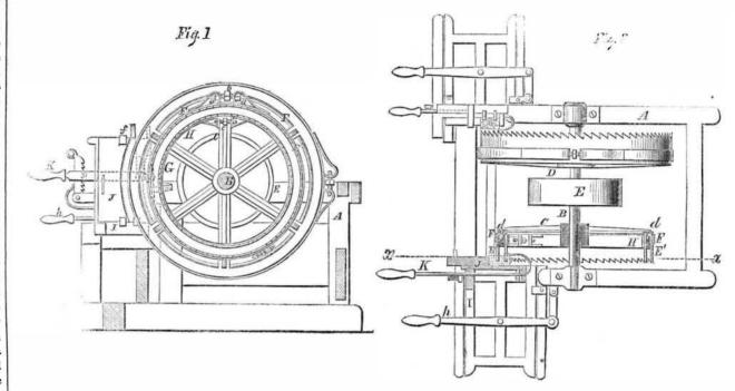
carriage, I, towards the saws by means of the lever, h. The two saws cut the fellies from the bolt exactly the shape they are required to be, and the thickness of the felly must depend on the number of rims between the saw, E', and the wheel, C, and fellies for wheels of different
