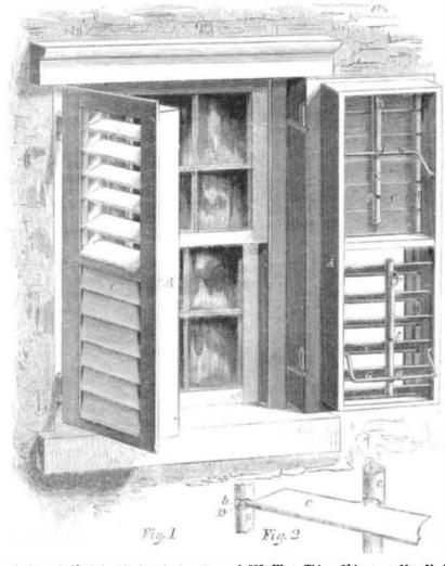
in the lower half of the blind, and when they are to be kept shut, it will fit into f, as seen the upper half, the sliding wire will be pushed over it, and it is most securely fixed. The principle offastening and attaching the slats can be equally as well applied to wood as iron, the advantage of iron being that it is fire and burglar proof.
