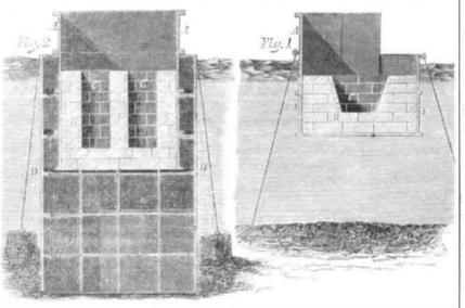
the London Engineer) relates to a mode of simplifying the construction of foundations of piers, harbors and other submarine structures. To attain this end, a floating caisson is formed of plates of cast or wrought iron, bolted or riveted together, and this floating vessel (which is open at the upper part) is brought over the spot which is intended to receive a
