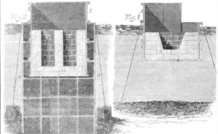
the London Engineer) relates to a mode of simplifying the construction of foundations of piers, harbors and other submarine structures. To attain this end, a floating caisson is formed of plates of cast or wrought iron, bolted or riveted together, and this floating vessel (which is open at the upper part) is brought over the spot which is intended to receive a
