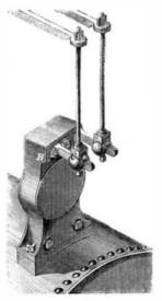
are more or less objectionable, on account of the springs becoming stiffer as the valve rises. Various plans have been adopted to overcome the defect by regulating the strength of the springs, thereby depending on the vigilance of the engineer to prevent the pressure from getting too great; whereas, the balance here illustrated, requires no attention whatever when in use, as an increase over the allotted pressure cannot take place
