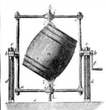
side, which are fitted in suitable bearings, c c, carried by A-shaped standards, dd, which are erected and rigidly fixed on the base or floor,
