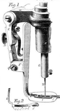
The mode of operation is as follows :- The it a piece, B, to which is hinged the piece, C, by the screw, c. The screw, D, fastens E, and to it is hinged by the screw, f, the foot, F; uppermost, and water or other fluid, with or this is kept on the cloth by the pressure of the
