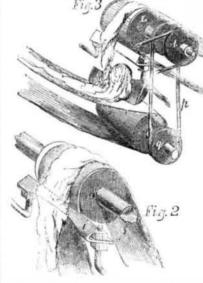
endless belt, G, being by it conveyed over the roller, L, seen in Fig. 3, when the scraper cuts it off, and lets it fall onto the endless band, H, which again conveys it into the mixer, C, from which it is taken by the endless belt, I,
