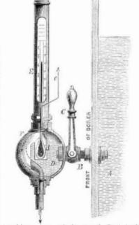
breaking. Part of the vessel, D, is broken away, to show the interior. E is the scale, and F a waste pipe, so placed that the excess steam or water can escape, and so allow the water in D to remain at its normal pressure; that is, at the same pressure as that in the boiler.
