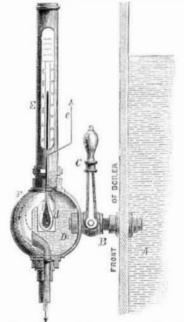
breaking. Part of the vessel, D, is broken away, to show the interior. E is the scale, and F a waste pipe, so placed that the excess steam or water can escape, and so allow the water in D to remain at its normal pressure: that is, at the same pressure as that in the
