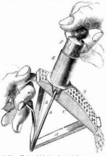
holder, E, in which it plays, being prevented from dropping out or touching the grater, by means of a short pin, projecting through a longitudinal slot in the holder, said pin and slot being so arranged that the piston may be entirely withdrawn from the cylinder whenever the operator wishes to insert an article to be grated. The method of holding the instrument in the hands and operating it is sufficiently explained by the engravings.
