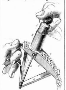
holder, E, in which it plays, being prevented from dropping out or touching the grater, by means of a short pin, projecting through a longitudinal slot in the holder, said pin and slot being so arranged that the piston may be entirely withdrawn from the cylinder whenever the operator wishes to insert an article to be grated. The method of holding the instrument in the hands and operating it is sufficiently explained by the engravings.
