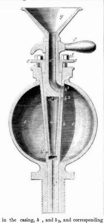
weather the holes,  $a^2$ , and a, in the plug, a. Only one of the holes or passages in the plug, a, need be in communication with the receiver at the same time, and each may be brought in communication by turning the handle, f, to the required position. In one position the steam entering the hollow of the plug will pass through the holes,  $a^2$ , and  $b^2$ , into the upper part of the receiver; in another position the lubricating matter will pass from the receiver
