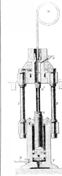
The manufacture of lead pipe by the ordinary method combines, like that of sheet lead, the double process of casting and elongation. Whatever may be the dimensions of shank is released, and the india rubber band the pipe required, it is first cast in the form
