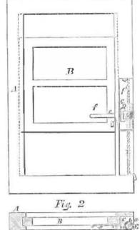
recess, f', in the frame, is placed the cord, E and to the side of B is attached the metal plate, C, whose outer edge is scen at a; another plate, D, is attached to it by an india rubber band, b, which passes through openings, c, in the plate. The outer edge of D is rounded, and the other has a shank, f, attached, which passes through a groove, e, in the stile of the sash.
