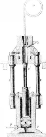
The manufacture of lead pipe by the ordinary method combines, like that of sheet lead, the double process of casting and elongation. Whatever may be the dimensions of shank is released, and the india rubber band the pipe required, it is first east in the form
