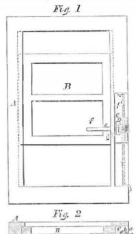
recess, f', in the frame, is placed the cord, E and to the side of B is attached the metal plate, C, whose outer edge is seen at a; another plate, D, is attached to it by an india rubber band, b, which passes through openings, c, in the plate. The outer edge of D is rounded, and the other has a shank, f, attached, which passes through a groove, e, in the stile of the
