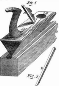
The plane stock, A, it will be seen, is made of triangular shape, and the cutting tool, B, which is quite narrow, projects at the apex of the angle. The plane is moved like the ordinary tool.
