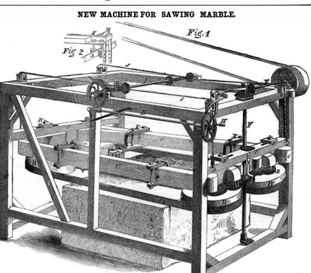
told that this machine cuts about three times | and there is no appreciable wear on their sur- | and operates with entire success. Further infaster than the common marble sawing appa- face. No difficulty is experienced in feeding ratuses. The endless saws may be driven at in the sand.
