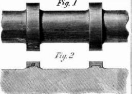
deal of trouble. A very neat way of putting them on by shrinking is shown in the accompanying engravings, in which Fig. 1 is a front elevation, and Fig. 2 a profile in section. The shaft is left slightly large where the journals occur, and bosses turned for the
