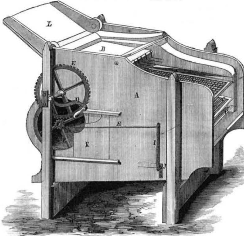
the frame. H is a rod connecting I with a any desired extent to regulate the supply of crank on the fan shaft, as represented. K is air to the fan, and consequently to increase a door which may be opened and closed to or diminish the blast through between the
