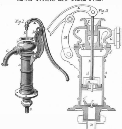
The pump represented in the accompany- | necessity for scarcely a single bolt. ing engravings is remarkable principally for | Fig. 1 is a perspective view from a dastrength, cheapness and durability. It is a guerreotype. Fig. 2 is a section copied from reciprocating pump, with valved bucket, like the Letters Patent. A is the barrel, and A' many of the most successful pumps previously an extension which is of larger diameter, and
