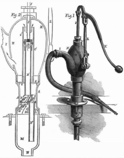
and allow the water to rise from M to fill the from the tube, B", and finally through the space. Whichever direction, therefore, the pipe or goose neck, I. bucket, B, is moved, the water rises from N into M, and proceeds almost directly there- further information address the inventor and from, either through B' or D, to be discharged patentee, Silas Hewit, Seneca Falls, N. Y.
