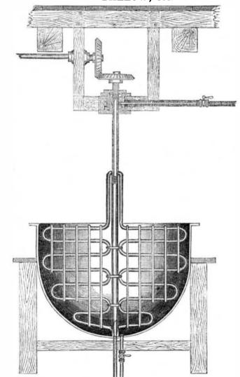
recently invented by Campbell Morfit, of Bal- | place co-incidently. timore, Md., for the simultaneous mixing and heating of compounds. It consists of an upright shaft with tubular arms or branches, and derives motion by means of cog-gearing from a steam engine. A stuffing box, near the top of the shaft and connecting the steam
