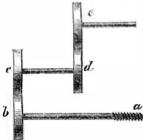
of threads to the inch on the lead or feed screw; b=the number of teeth on the screw wheel; c=the number of teeth on the loose wheel of the stud spindle: d= the number of teeth on the fast wheel of the stud spindle ;
