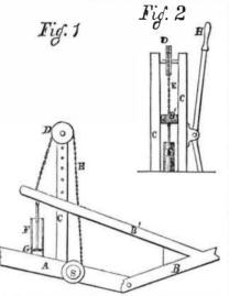
F, is attached to the under side of the arm B by a flexible joint or hinge and is provided with a valve on its lower side, said valve opening downwards. H is a clutch lever suspended by a suitable joint from standards C C.
