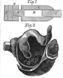
der, and C is an iron plug fitted in the opening. To the stub, D, is fitted a sabot of cork, E, with two pieces of leather, F, glued to it. The sabot is made of greater diameter than the ball. If employed for a rifled cannon, the elongated shot, A, of cast iron, can be used without injuring the grooves of the gun, as the sabot will fill the grooves and receive the spiral motion in its discharge.
