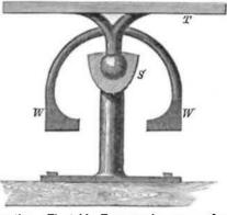
motion. The table, T, moves by means of a ball fixed in the socket, S, which is fastened to the deck. W W are weights which preserve it in a horizontal position. The same principle, heurges, would of course apply to many forms.
