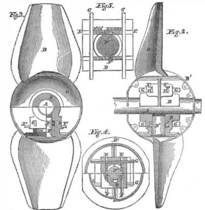
drical portion D' shall correspond with the grooves in the opposite sides of the cylindrical cavity in the solid hub, into which it is to be inserted. To allow the blade to be revolved after it is fairly in its place, an annular space or ring of sufficient size is turned out. It is now easy to see that the blade can be inserted only when held in one position ; but after it is fairly in its place in the hub, it can be readily turned into any position desired.
