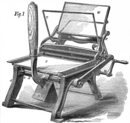
as to produce a very powerful impression on | O are drawn again across the form, inking it the form. On lifting I, all the motions are for a new impression. As the platen E recedes reversed, the levers G move backward, acting into the position represented in Fig. 1, it on H, to elevate the platen E, and while these leaves the frisket T in the position indicated, parts are returning to their places, the rollers and allows the printed sheet to be readily
