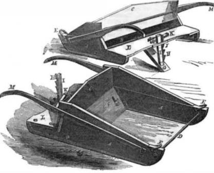
etc. For some, perhaps for most, purposes. it is desirable to give a curved outline to the lower edge of F, so that the shallow channel excavated shall have in no case any perpendicular sides. The implement seems very Ohio.
