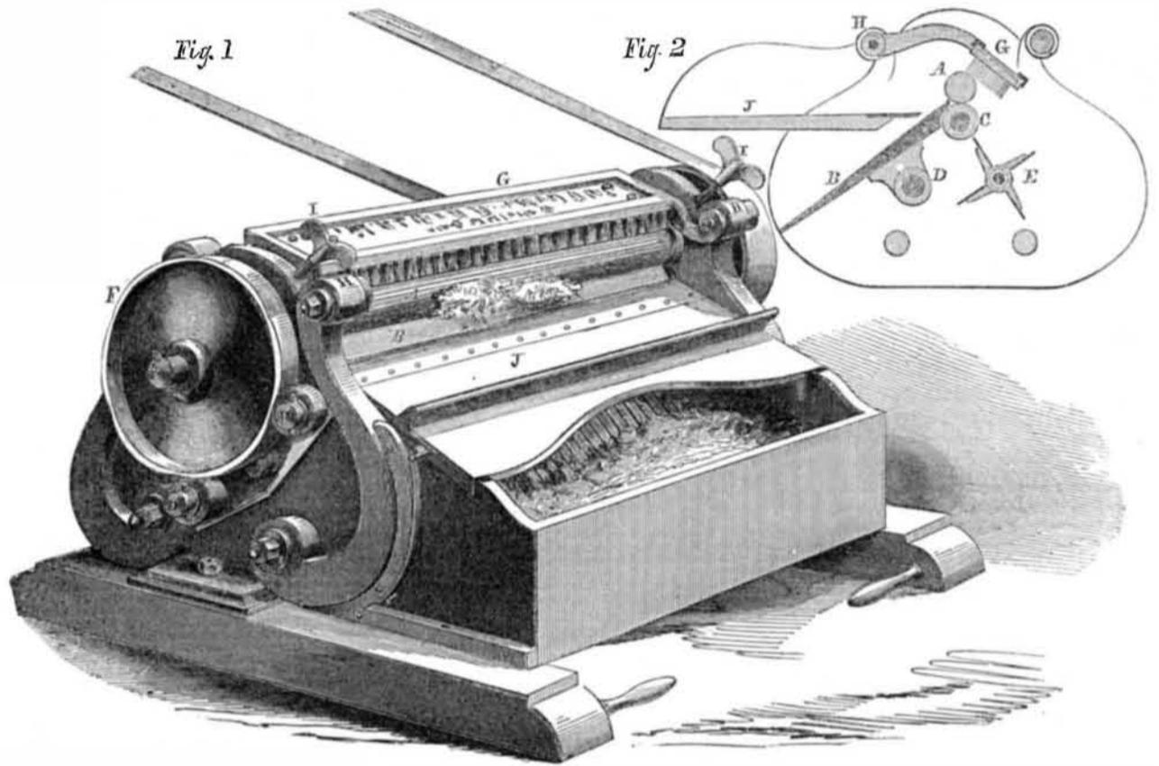
crushing of the seeds. The difficulties incident to the use of these gins are quite numerous, not the least of which is the very serious tendency to take fire from friction; and the bearings are almost invariably changed to charcoal in a very short time.
