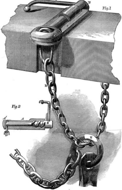
Holmes, of this city, on the 28th of April last, for the easy, rapid and safe release of an anchor when it is desired to let it fall. It is shown in perspective by Fig. 1, and in longitudinal section on a smaller scale by Fig. 2.
