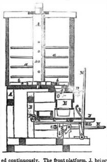
ed continuously. The front platform, J, being pivoted, if stones should get into the molds with the clay, and project above their upper surface, this platform can be lowered to allow the molds to be discharged.
