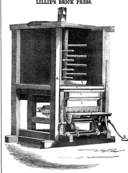
racks, *i*, forcing the empty mold and box, E, upwards into box C. The mold box is thus filled: the clay being forced through the grate, F, into the several molds in one box, the box E acting as a plunger. When pressure is removed from the treddle, H, the box, molds, and platform, descend by their own gravity. The lever, M, is then raised to the positionshown, and the same operations repeat-
