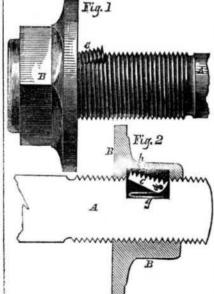
The incessant action to which such fastenings are exposed, the necessary looseness to allow of the revolution and a slight end play of the wheels, and the serious consequences liable to accrue from a sudden loss of a wheel in rapid traveling, gives great importance to the subject, and we take pleasure in giving publicity to the ingenious device under consideration as one entitled to especial attention
