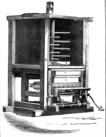
racks, i, forcing the empty mold and box, E, upwards into box C. The mold box is thus filled: the clay being forced through the grate, F, into the several molds in one box, the box E acting as a plunger. When pressure is removed from the treddle, H, the box, molds, and platform, descend by their own gravity. The lever, M, is then raised to the positionshown, and the same operations repeat-
