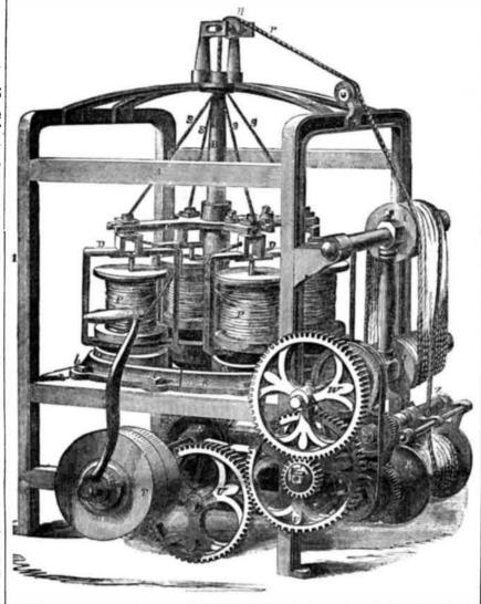
view of the improved rope-making machine, for which a patent was issued to Milton Wallwork on the 7th of April last. The improvement relates to the "sun and planet" rope machine, and consists in the means of controlling the speed of the strand flyers, for enabling the twist of the strands to be varied with facility. The figure represents the application of the machine to laying rope in a very small space, obviating the use of long rope walks.
