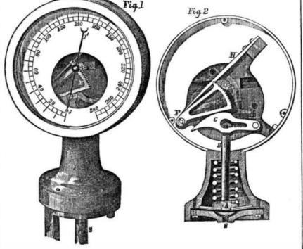
means indicates exactly the pressure. H is a | portion of the face of the dial is left open as slender spring, which acts on E with sufficient | represented, in order to see that all the parts intensity to overcome the slight friction and insure its falling back, whenever the pressure mounted in a block, so that it may be traof the steam is lowered and B is depressed by versed in a groove across the gage, to facilithe action of the stout coiled spring.
