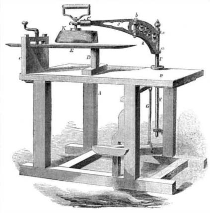
to any extent desired. This allows of an | the joint, C', where the swivel, C, is attached easy motion in every direction horizontally, while by the aid of the link, G, forming a connection between the treadle and the rod, F, a degree of pressure for any kind of tailors' work is obtained without difficulty, and in a manner very easy for the operator.
