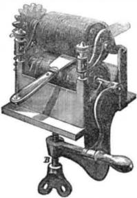
rollers. In order to scour a knife with this machine, it is only necessary to fill the trough with some suitable cleansing material.
