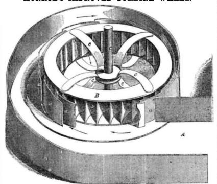
The accompanying figure is a perspective | scroll for conducting the water, and B is the The improvement in this class of wheels conguide plates in the scroll, for the purpose of causing the water to act in the proper direction against the buckets. The buckets are concave, and the central arms are inclined plates, which tend to a more free discharge of the water from the wheel to relieve it, after the water has acted on the buckets.
