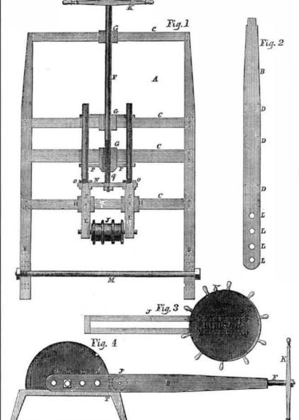
F, figure 1, is a regulating rod passing through while the machine is revolving, to turn the a threaded slide nut, G, a corresponding thread | lever wheel, K, in order always to keep the being cut on the rod, by which means the timber firmly pressed against the mold, by bending roller is raised or lowered by turning the hand wheel, K. S S, figure 1, represent thumb set screws, which prevent all lateral play of the slides and bending roller while the timber is being bent.
