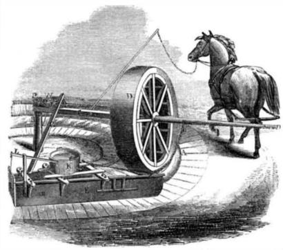
down, the drag then gathers the mortar | form us, that with the labor of one man and formed into a heap, if desired, or pushes it a horse, thirty casks of lime can be made a trap door in path A. The lime employed is previously slacked before it is put on the way, A. A few revolutions of the roller and drag mixes the materials.
