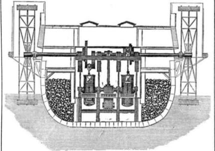
common on most of our ocean steamers, but by four engines coupled in pairs, one pair for each paddle wheel; but the main shafts and wheels, though thus capable of working independently—so that one may be worked while the other is idle, or both may be worked in opposite directions if desired, Mississippi steamboat fashion-are to be coupled or uncoupled at pleasure by a strong friction clutch. 'eet-as great, we think, as any in the world, the center of the mammoth hull.
