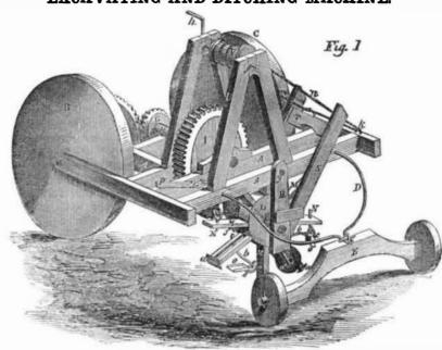
may be disconnected from springs, d, and ataction, and the scoops so arranged will cast their contents by the centrifugal action of the excavating wheel in a regular line, as the machine is drawn along. When the lifted earth is to be scattered at the side promiscuously, the scoops have different inclinations to discharge at different points of their circuit.
