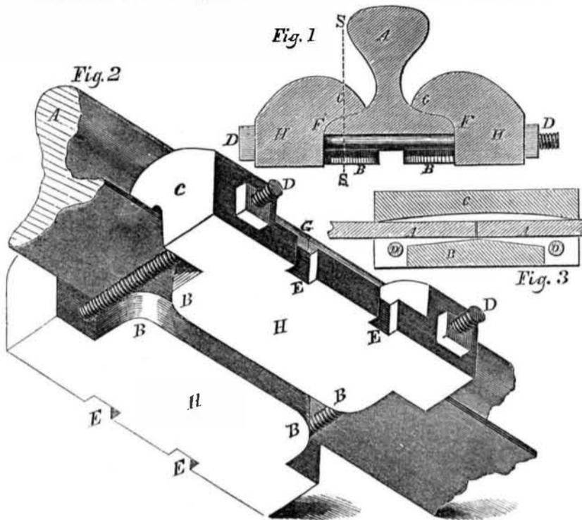
braces the joint so as to prevent its settling under the weight of the heaviest engine, and this, too, on an unballasted road bed. The battering of the ends of the rails, which takes place with most chairs now in use, is effectually prevented by this one, as it renders any considerable working or sinking of the ends of one rail below its fellow impossible. These
