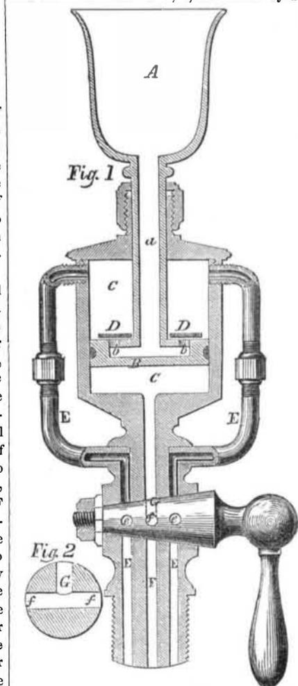
somewhat enlarged cross section of the cock in figure 2) allows the escape of the steam from the lower portion of C, through a side opening, and both sides of B being now sub-
